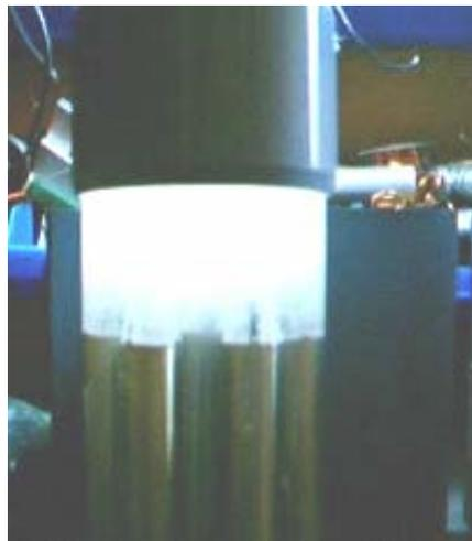
The mounting rings for the tubes can be made from any suitable plastic, such as that used for ordinary food-chopping boards, and are shaped like this:
